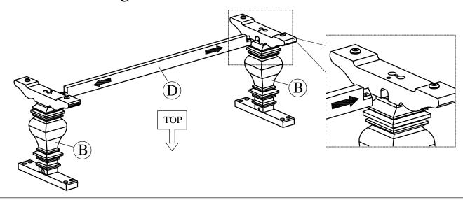
Using a second person to assist you, place both Leg Posts (B) upside down onto a padded, non-marring surface as shown. Insert Bottom Stretcher (D) into the corresponding notched hole in the bottom of Leg Post (B).
