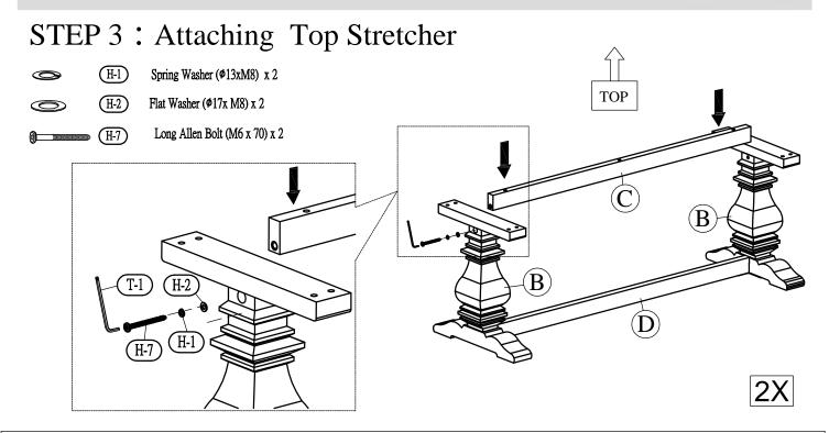
Using a second person to assist you, turn the assembly (from Step 2) upright as shown. Attach Top Stretcher (C) to both Leg Posts (B) and secure using Long Allen Bolts (H-7), Spring Washers (H-1) and Flat Washers (H-2), stacking the hardware in the order shown. Engage bolts by hand but do not fully tighten them yet.
